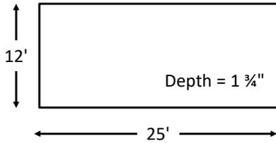
$$\frac{25'}{\text{Length}} \times \frac{12'}{\text{Width}} \times \frac{0.14'}{\text{Depth}} = \underline{42 \text{ Cubic Feet}} \text{ Volume}$$
