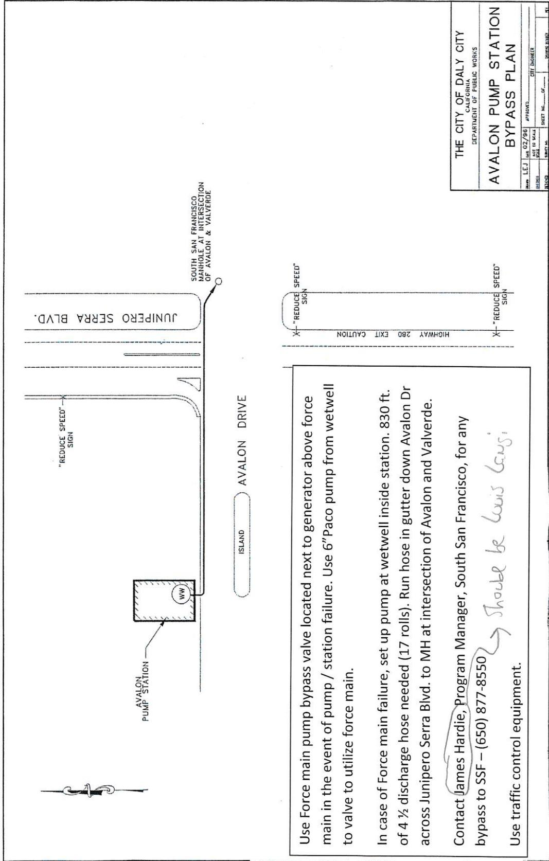
Use Force main pump bypass valve located next to generator above force main in the event of pump / station failure. Use 6" Paco pump from wetwell to valve to utilize force main.
