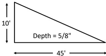
$$0.5 \times \frac{45'}{\text{Base}} \times \frac{10'}{\text{Height}} \times \frac{0.05'}{\text{Depth}} \times \frac{7.48}{\text{gal/ft}^3} = \underline{84.15 \text{ gallons}} \text{ Volume}$$
