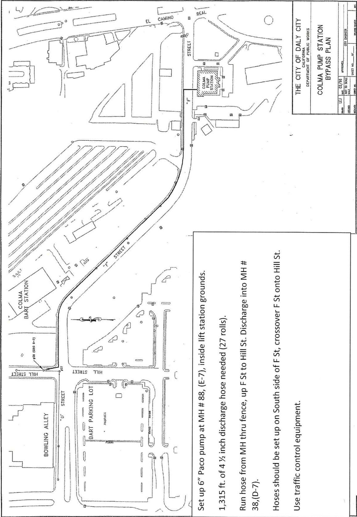
Set up 6" Paco pump at MH # 88, (E-7), inside lift station grounds.
