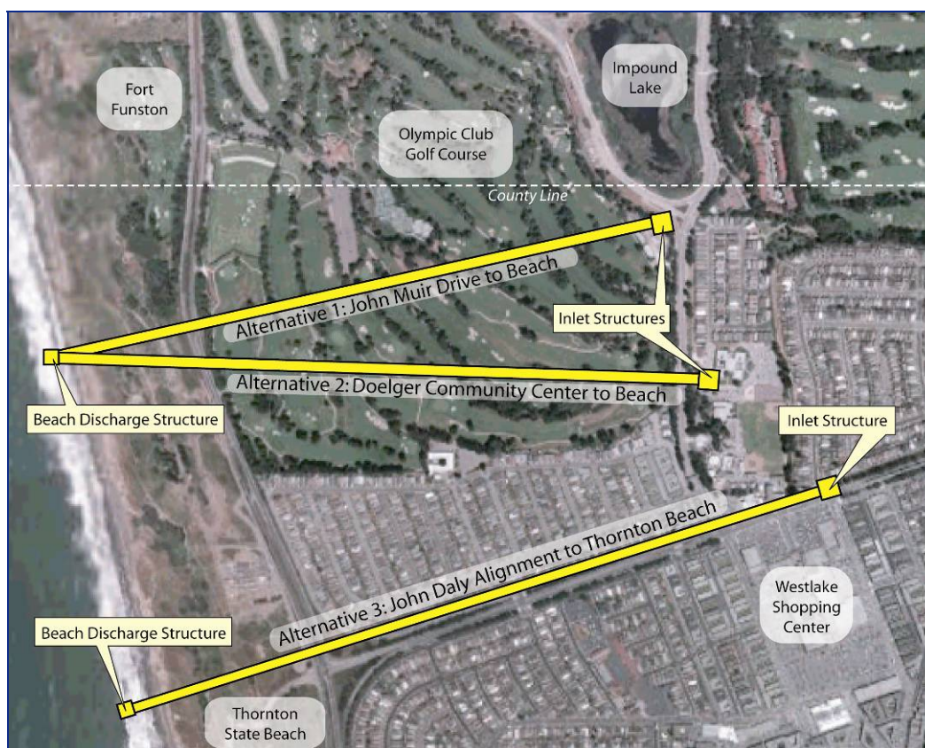
Figure 5-2 Tunnel South of County Line Alternative Map
