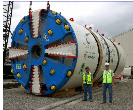
Figure 5-4 Typical tunnel boring machine
