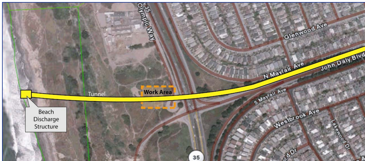
Figure 5-14: John Daly Alignment Primary Construction Site
