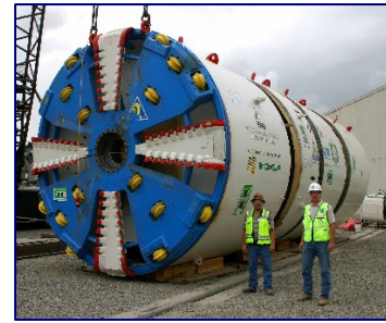
Figure ES-12 Typical Tunnel Boring Machine
