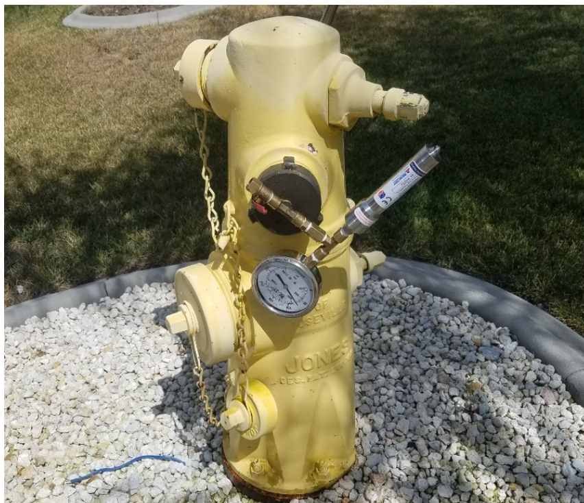
Figure 2-1. Pressure gauge and logger connected to the pressure hydrant
