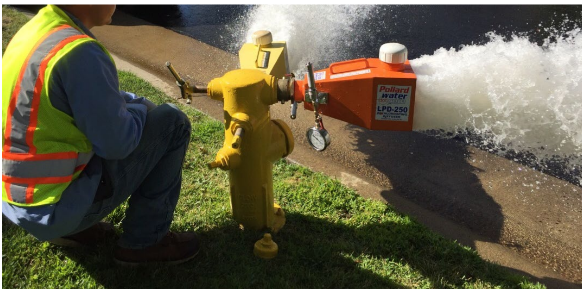
Figure 2-2. One or two flow diffusers connected to the flow hydrant
